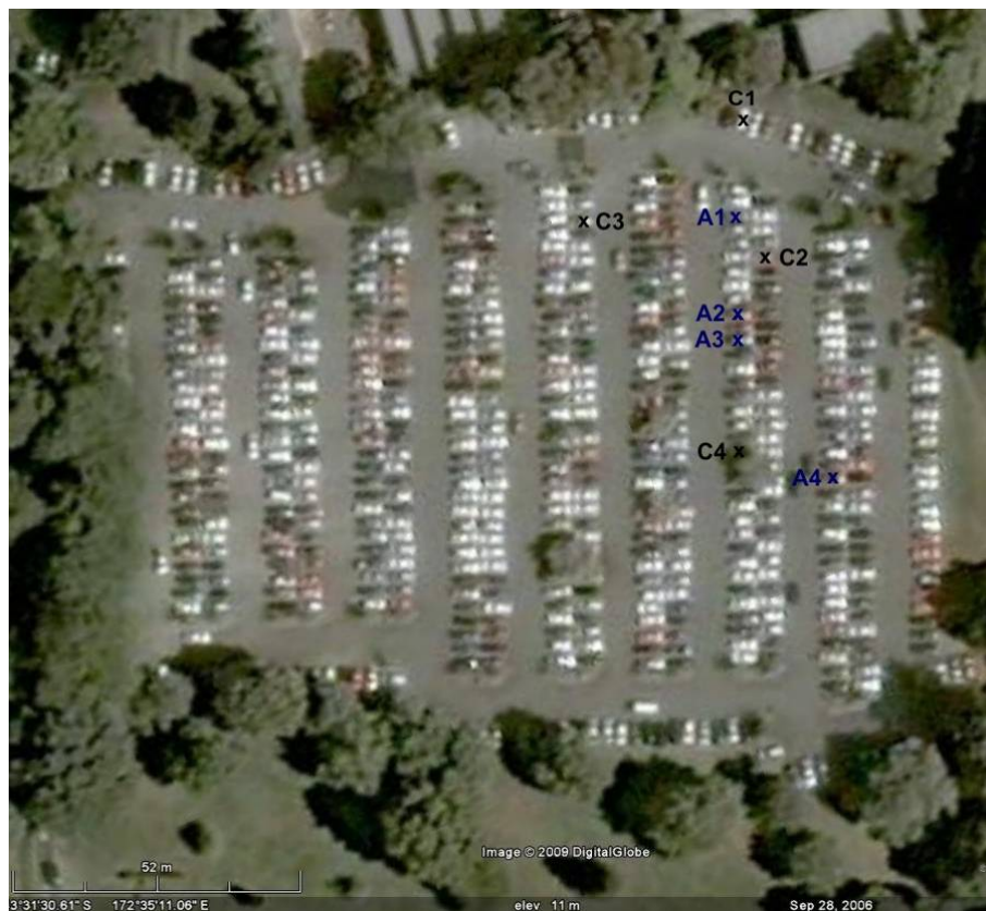
Fig. 1: Position of boards placed on the carpark: A1-A4 – asphalt boards, C1-C4: concrete boards. Main carpark entrance is in the upper right corner.
