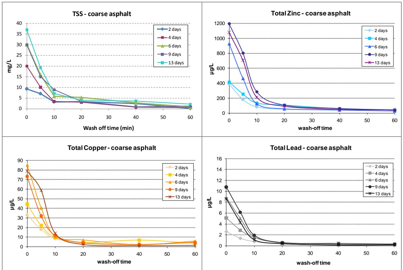
**Figure 5:** TSS, Zn, Cu and Pb concentrations in runoff from coarse (14 mm aggregate) asphalt boards using a rainfall simulator at a rain intensity of 22 mm/h after exposure at a carpark for 2 – 13 days.
