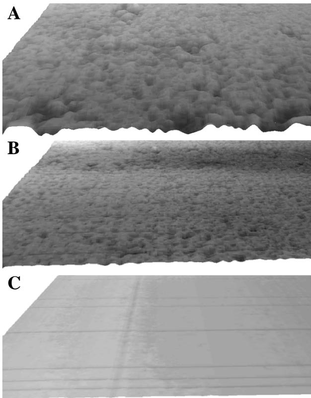
**Figure 1:** Three-dimensional images of different board types as derived from surface laser scanner. A – coarse asphalt, B – fine asphalt, C – concrete. Heights are represented by differences in grey levels with dark tones showing lower elevations.
