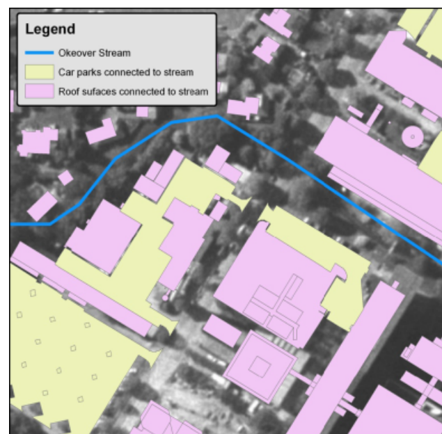
Figure 5 | Impermeable surfaces directly feeding runoff to the urban waterway used for modelling purposes and for demonstrating contaminants origins.
